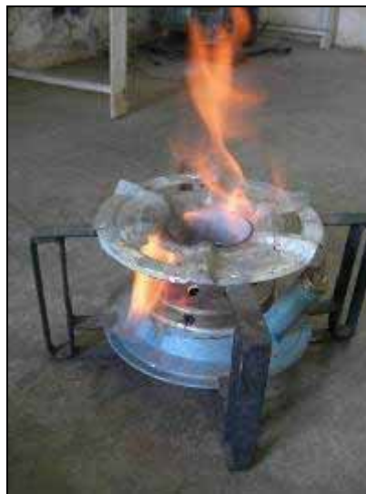
A blocked fuel return pipe causes the burner cup to overflow, spilling fuel which then ignites
