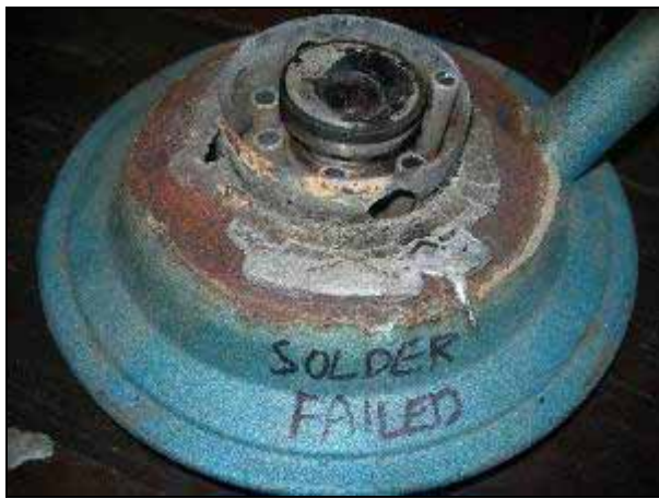
Stove with solder failure between the burner cup and tank (the holes in the tank occurred during the removal of the regulator)
