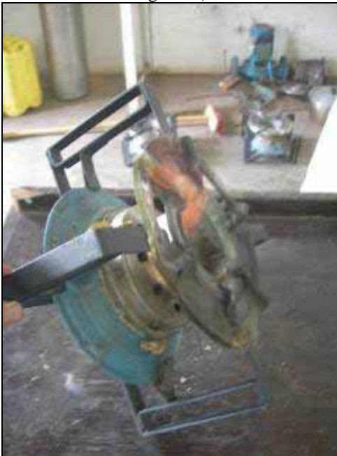
Stove tipping angle – note the continued operation of the stove and the stable flame
