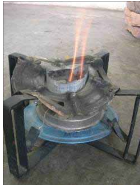
Just before the end of the destruction test – the stove was still working despite the application of a large metal bar.
