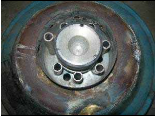
Stove with oversized nozzle preheat holes
