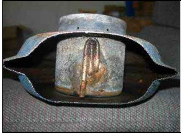
Stove post mortem showing tank deposits and incorrect fuel pipe/tank geometry
