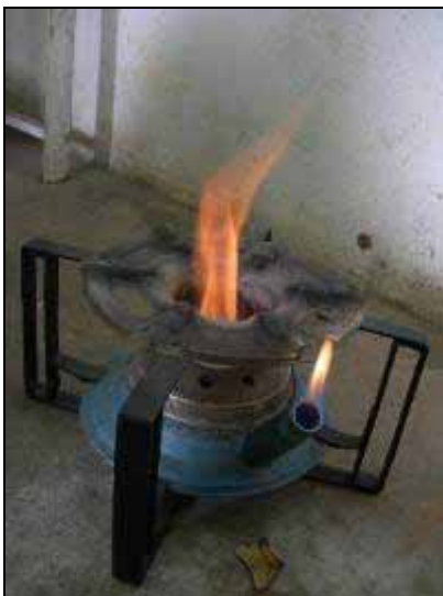
With the fuel cap left off and the stove shaken a small steady flame appears at the fuel tank inlet
