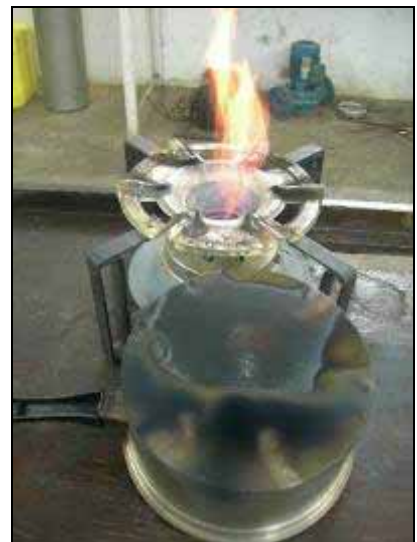
Soot deposits on a pot base from a typical WBT phase
