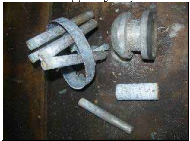
Oxide build up (?) inside the burner cup (the damage occurred during the removal of the components)
