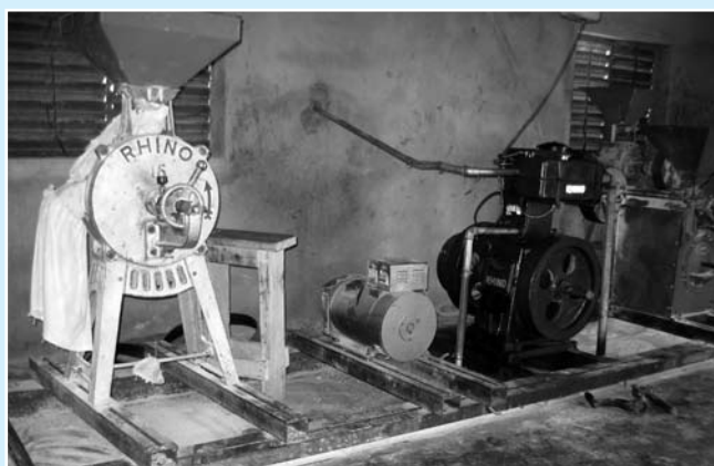
Figure 12 A multi-functional platform that runs on diesel or liquid biofuels, and can be used for maize milling as well as electricity production. (Photo: PREDAS)
