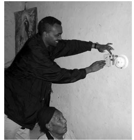
Figure 1 (above). Gaia Association enumerator, Yonas Abesha installing indoor air quality monitoring equipment (UCB, HOB0 and CO tube) in an Addis Ababa kitchen. (Photo: Amdework Wbetu)
