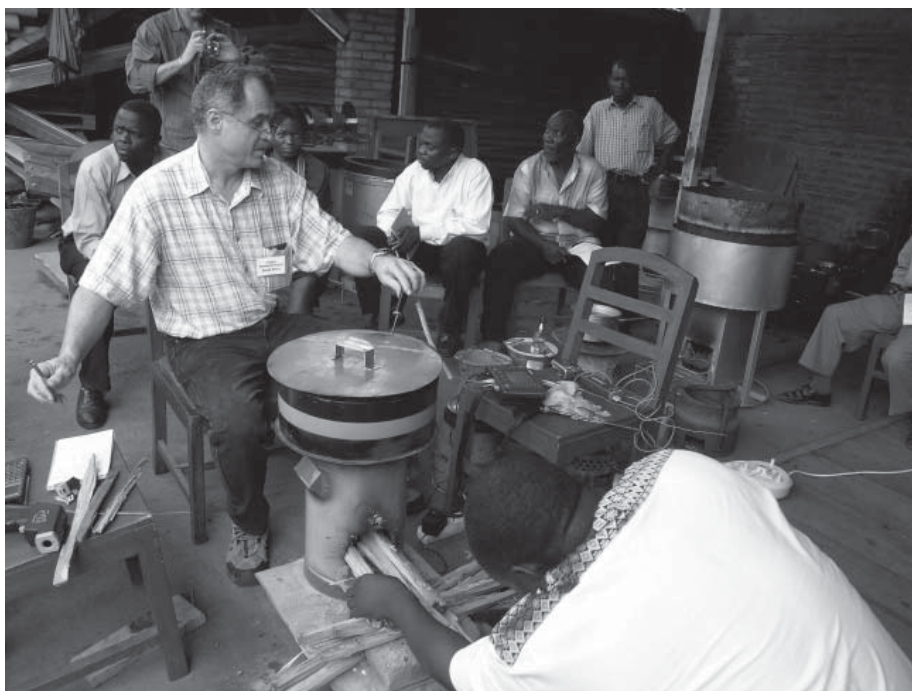
Figure 1 Testing of a commercially manufactured Rocket Stove from Uganda, at GTZ Technical Workshop in Mulanje, Malawi (photo: Elmar Dimpl)
