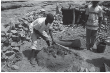
Figure 3 After one week the mix is ready to be used for the fabrication of the stove. (photo: Peeyush Sekhsaria)
