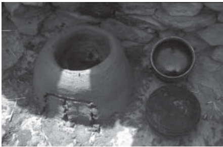
Figure 9 The opening for firewood is marked in the moist earth. The opening will be removed after a day. (photo: Peeyush Sekhsaria)
