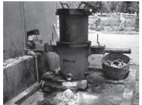
Figure 2 Updraft gasifier for cooking (photo: Dr Sanjay Mande & Debajit Palit)
