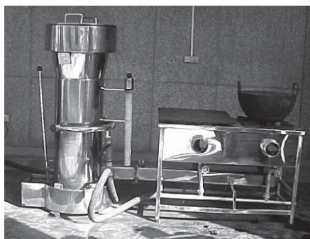
Figure 1 Downdraft gasifier for cooking (photo: Dr Sanjay Mande & Debajit Palit)
