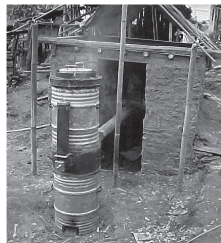
Figure 3 Gasifier for cardamom drying (photo: Dr Sanjay Mande & Debajit Palit)
