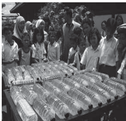
Figure 4 The water bottles can also be placed on a corrugated iron sheet (photo: Yayasan Dian Desa, Yogyakarta, Indonesia)
