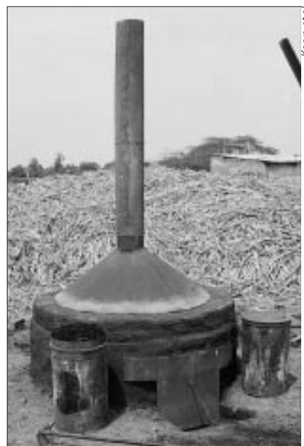
Figure 2: Prototype kiln at ARTI's field station in Phaltan, Maharashtra State
