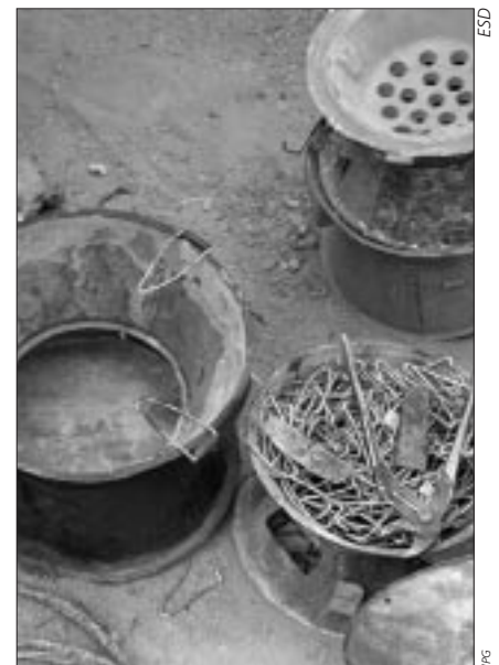
Figure 1: Lakech charcoal stove under construction
