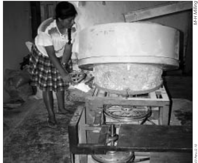
Figure 1: Production technology to reduce human drudgery; a woman using micro-hydro powered milling machine
